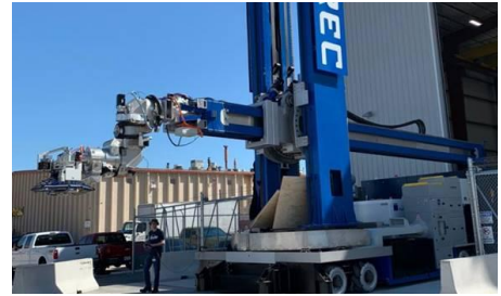
XYREC's robotic technology can measure over 72 feet when the arm is fully extended. Here, the large crane-mounted robot is positioned directly outside the company's new facility at Port San Antonio — XYREC'S first North American operation.
