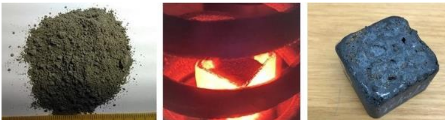
LEFT: Building blocks for extra-terrestrial colonization: Powdered basaltic matter is subjected to high temperatures in the research team's experimental vacuum oven and then molded into bricks to create building components for landing pads on the Moon and Mars. Image credit: Astroport Space Technologies/WEX Foundation.
