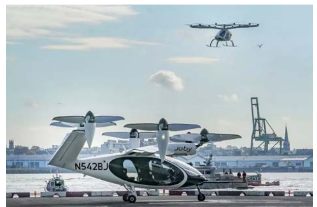
An electric vertical takeoff and landing — eVTOL — aircraft, flies above Joby eVTOLs on the tarmac in New York in this 2023 file photo. Bebetto Matthews/Associated Press file photo
