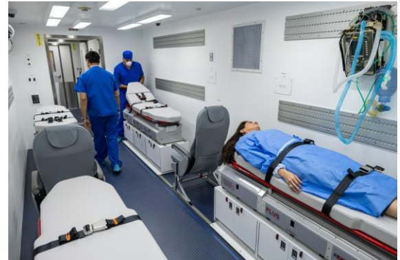
Knight Aerospace's aeromedical modules are rolled into the back of cargo aircraft, instantly converting them to flying medical facilities.
